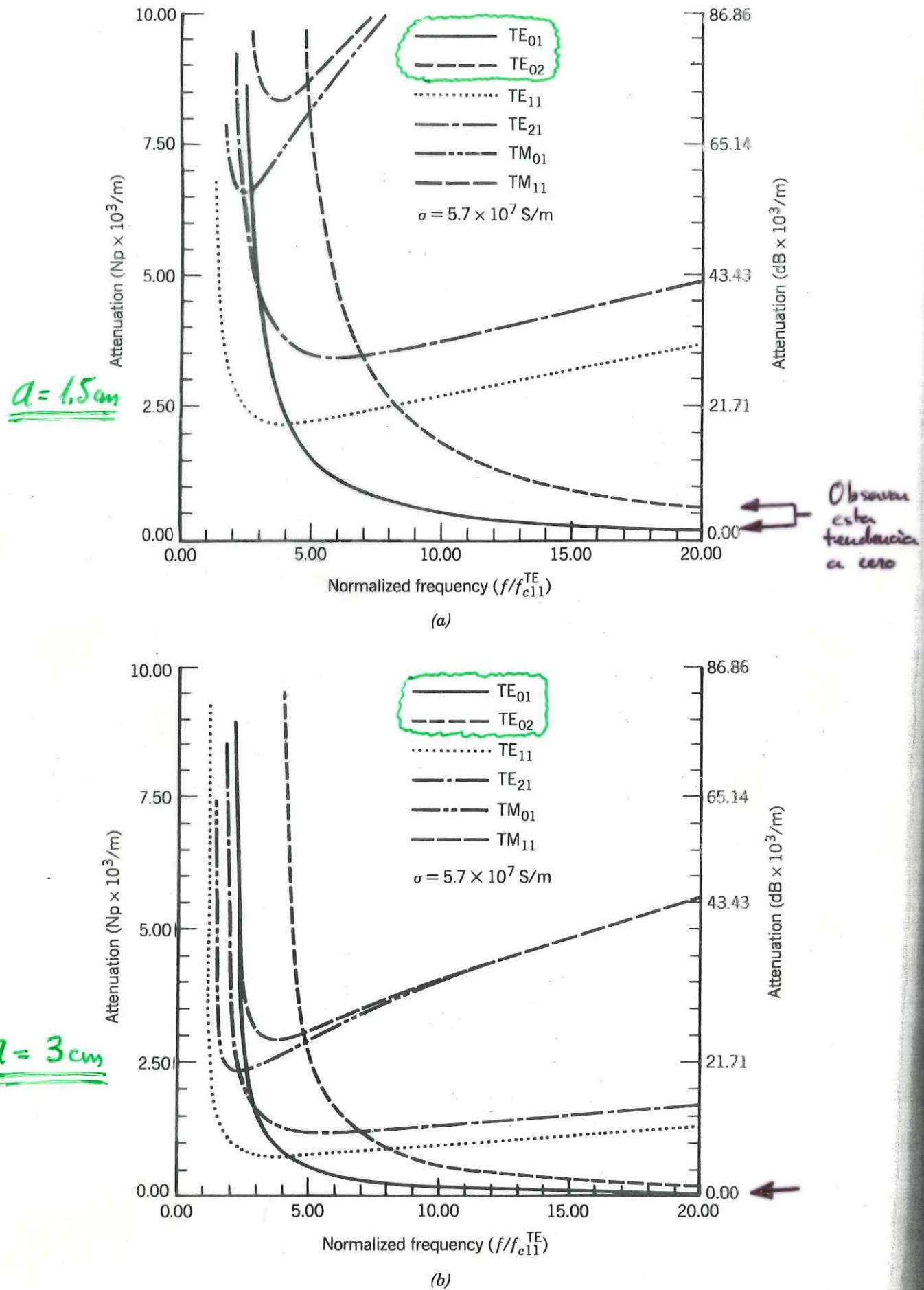
FIGURE 9-4 Attenuation for  $\text{TE}_{mn}^z$  and  $\text{TM}_{mn}^z$  modes in a circular waveguide. (a)  $a = 1.5 \text{ cm}$ . (b)  $a = 3 \text{ cm}$ .
