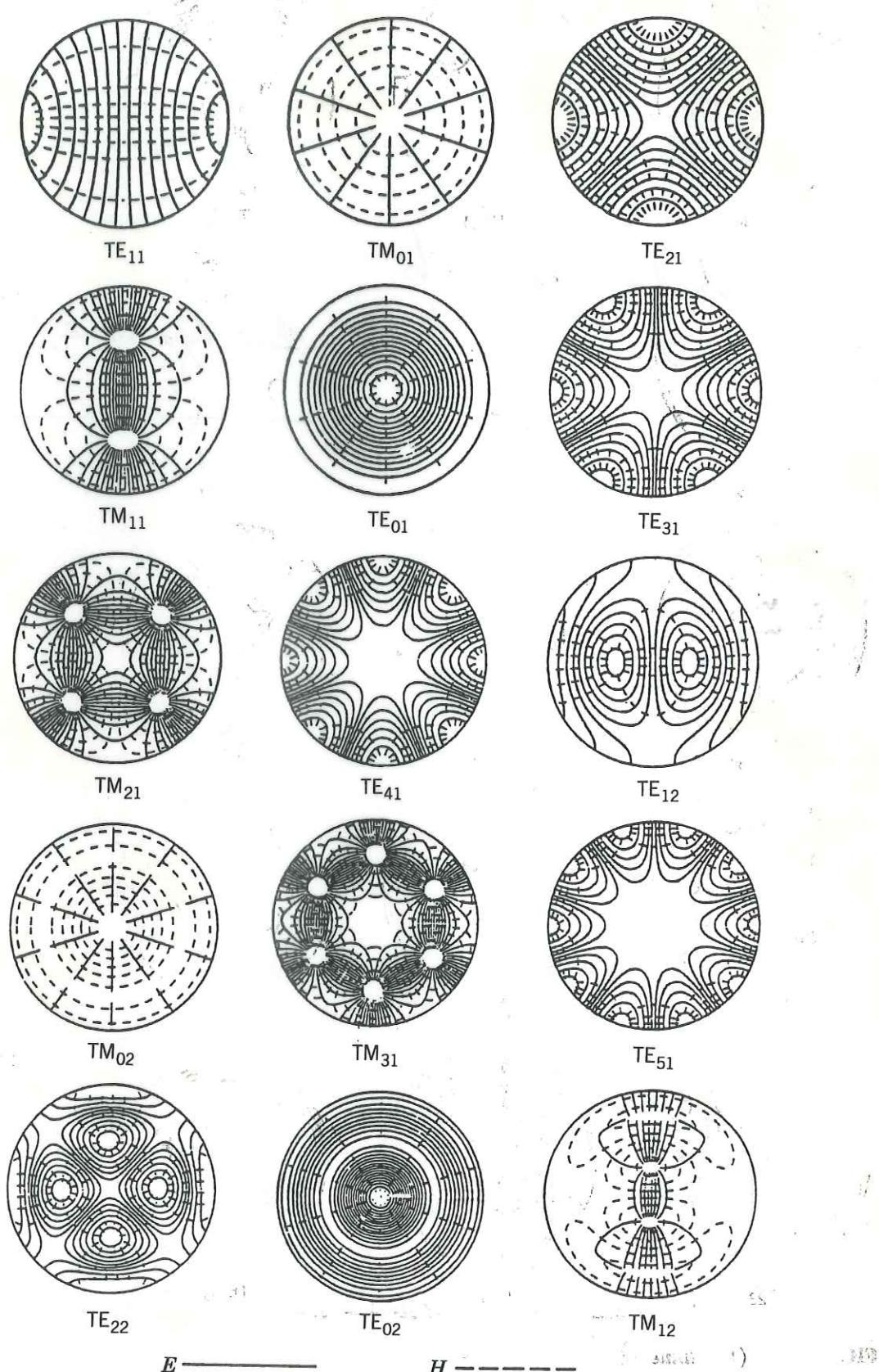
**FIGURE 9-2** Field configurations of first 30 TE<sup>z</sup> and/or TM<sup>z</sup> modes in a circular waveguide. (Source: C. S. Lee, S. W. Lee, and S. L. Chuang, "Plot of modal field distribution in rectangular and circular waveguides," *IEEE Trans. Microwave Theory Tech.*, © 1966, IEEE.)
